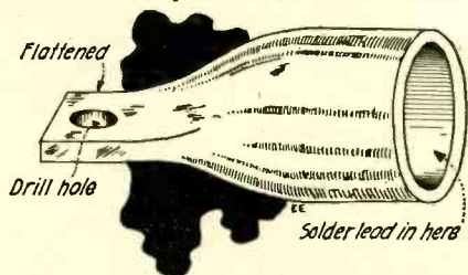
Good Wire Terminals or Lugs Can Be Fashioned from Copper Rifle Shells.
